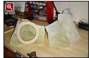
One mould with MDF-ring mounted. To the right you'll see how it is out of the car (but with the extra layer of glassfibre).
